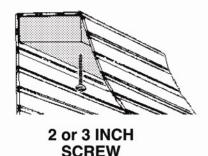
Note: Installation with 2" or 3" screws is intended for inside or ceiling mount only. No bracket is required.
