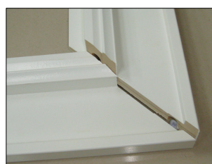
Position the left frame on the Hoffman Key and push down until the frames mitered edges are flush.
