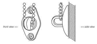
Install the Cord Guide such that the cord hangs loosely – this optimizes the performance of the clutch, and assures that the Cord Connector will pass through the Cord Guide with relative ease. Do not twist or cross the control cord/bead chain. In order to position the base properly, adjust the cord so that the Cord Guide is at the bottom of the cord loop and let it hang freely. Compress the spring by hand so that the chain moves freely through the 'U' channel.
