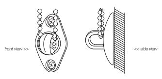
Install the Cord Guide such that the cord hangs loosely – this optimizes the performance of the clutch, and assures that the Cord Connector will pass through the Cord Guide with relative ease. Do not twist or cross the control cord/bead chain. In order to position the base properly, adjust the cord so that the Cord Guide is at the bottom of the cord loop and let it hang freely. Compress the spring by hand so that the chain moves freely through the 'U' channel.
